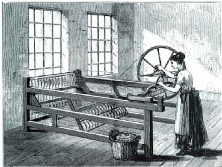
Hargreaves' spinning jenny, the first practical application of multiple spinning by a machine. The raw cotton was unwound from the vertical bobbins (left), pulled out and twisted, and the spun thread reeled onto the lower bobbins.
